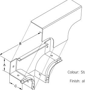
Notes: relating all products Material: UL94/V0, Zero Halogen. Colour: Standard yellow. Other colours on request. All dimensions are for reference only. Finish: all outside surfaces have a haircell texture. All parts have predrilled fastening holes. Dimensions in mm.
