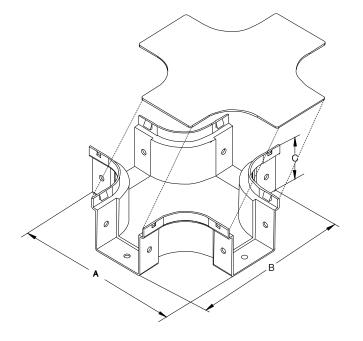
Notes: relating all products Material: UL94/V0, Zero Halogen. Colour: Standard yellow. Other colours on request. All dimensions are for reference only. Finish: all outside surfaces have a haircell texture. All parts have predrilled fastening holes. Dimensions in mm.
