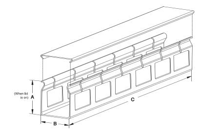
Cut out size: 50 x 50mm - 25mm (h) x 32mm(w) 100 x 100mm - 70mm (h) x 32mm(w)
