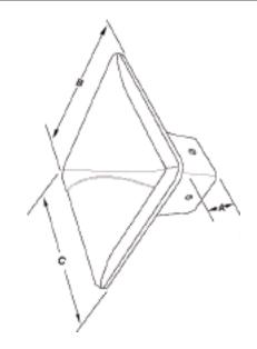
Notes: relating all products Material: UL94/V0, Zero Halogen. Colour: Standard yellow. Other colours on request. All dimensions are for reference only. Finish: all outside surfaces have a haircell texture. All parts have predrilled fastening holes. Dimensions in mm.
