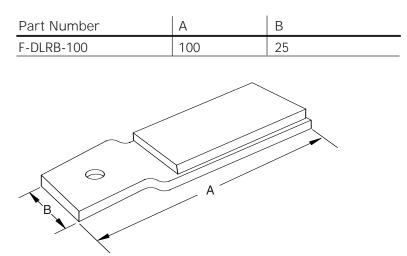
Material: Mild Steel, Zinc Plated and Passivated. All dimensions are for reference only. Dimensions in mm.
