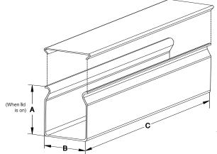
Material: UL94/V0, Zero Halogen. Colour: Standard yellow. Other colours on request. All dimensions are for reference only. Finish: Haircell Dimensions in mm.
